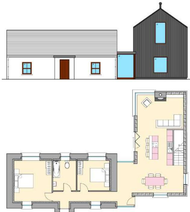
7. Space heating is provided in a family living area by a wood-burning stove inset into a chimney breast, as shown. The chimney has been constructed to accommodate the stove and is located on a 200 mm internal solid concrete block wall. A 150 mm diameter cast iron flue connects the stove to the chimney flue. The living area has an insulated solid concrete ground floor with a 20 mm hardwood finish. The dimensions of the stove are: height 600 mm, width 550 mm, depth 400 mm.
